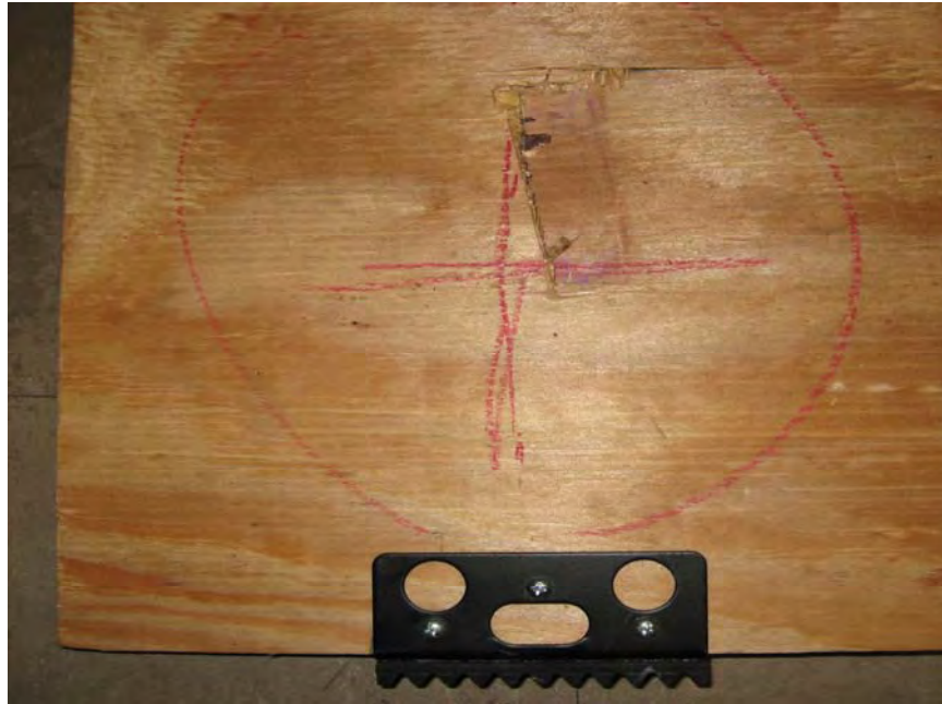
Photo No. 3 Specimen # 2 Lower Left Corner Impact
