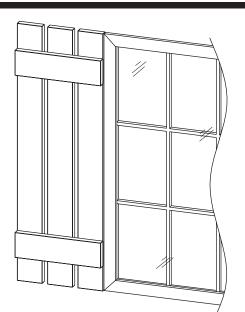
Note: If installing on masonry, transfer the holes in the shutter onto the wall. Using a masonry drill bit, drill the holes into the wall. Install the wall anchors according to the instructions supplied with them and install shutters.
